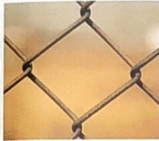
Aluminized Steel— 10% Pinpoint Rust, 90% Black*
